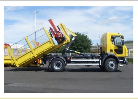
Innovative concept with tilting frame that is locked on the sub-frame in loading phase
